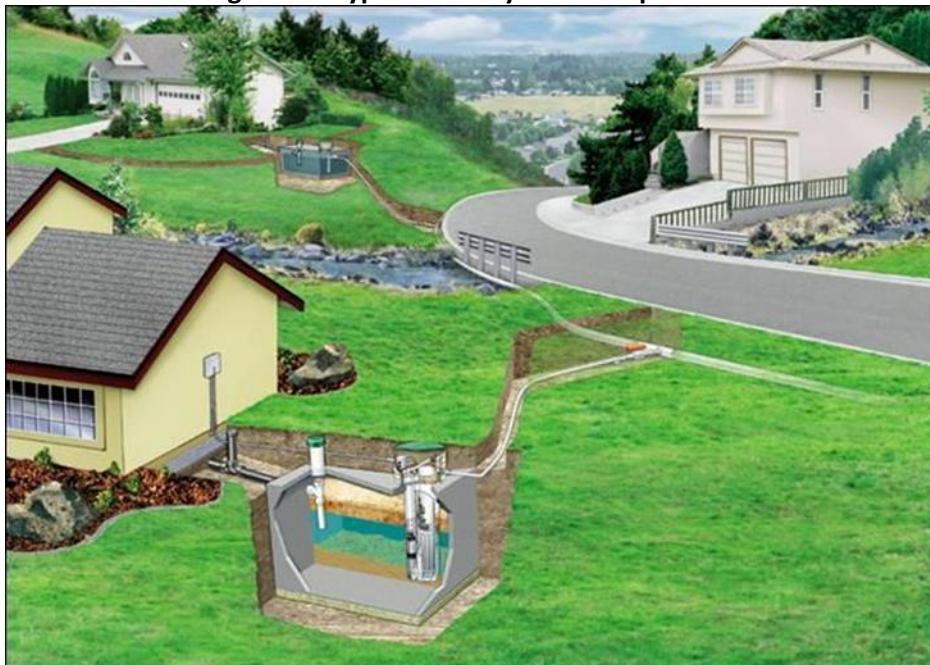
Figure 2: Typical STEP System Components
